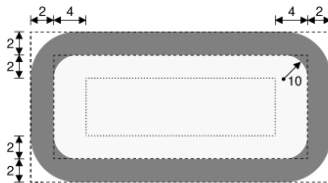
Figure 19.8. Structure of a QLineEdit
