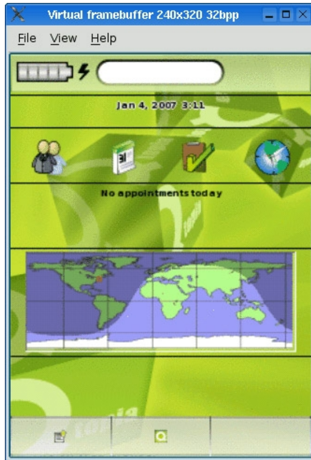
Figure 24.1. Qt/Embedded Linux running in a virtual framebuffer
