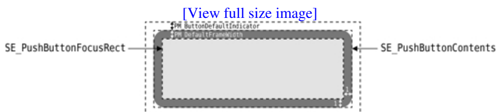
Figure 19.19. Structure of a QPushButton
